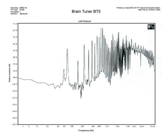
Fast Fourier Transform (FFT) Spectrum Analysis in the Frequency Domain of the original BT5
